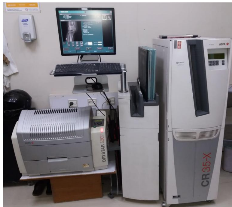
Figure 5: Agfa Fuji Computerized Radiography System, CR-35X showing foot print digitizer, Central Processing Unit and monitor (Radiology dept, Patel hospital, Karachi, 2018- 2019)
