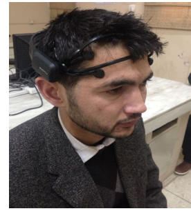
Fig. 2. Data Acquisition through Emotiv Sensor
