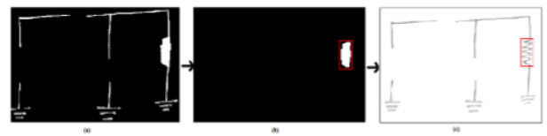
Fig. 4: Segmentation of components with connected lines: (a) Image after morphological closing (b) Removal of other components and detection of respective component (c) Localization of component in original image
