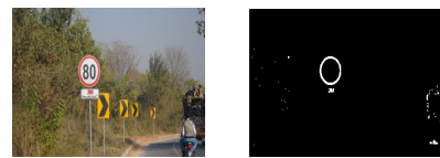
Figure 2: A road scene image and result of (red) color based thresholding
