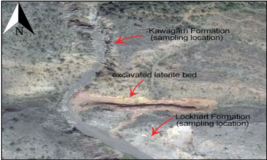
Figure 2.3. Satellite image showing Formations (sampling locations) and excavated Laterite bed (Google Earth).
