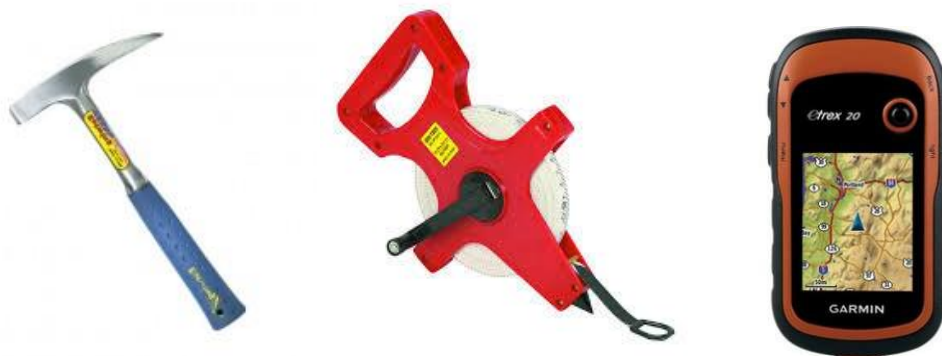
Figure 1.2. Field instruments, (A): Geological hammer (B): Measuring tape (C): GPS
