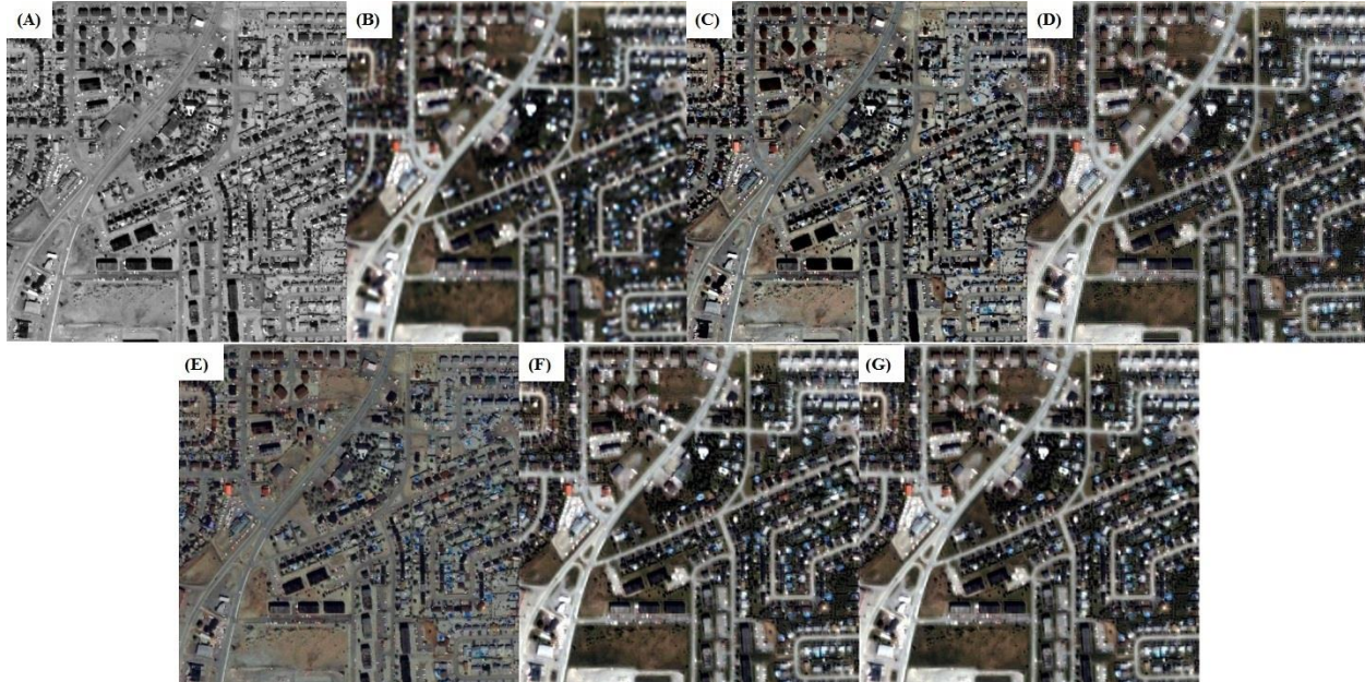
Figure 4.1: Visual Comparison of Experiment 1, P (1 m resolution, 0.45–0.90 \mu\text{m} ). MS [4 m resolution, blue (0.45–0.52 \mu\text{m} ), green (0.51–0.60 \mu\text{m} ), red (0.63–0.70 \mu\text{m} ), NIR (0.76–0.85 \mu\text{m} )] [2, 49]
