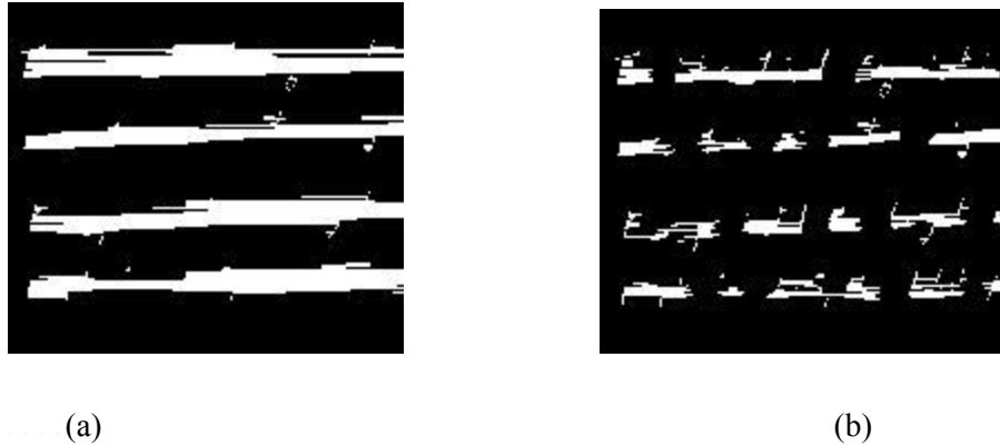
Figure 5.5: (a) Horizontal Run Length Smoothing Algorithm (a) Line Detection (b) Words Detection
