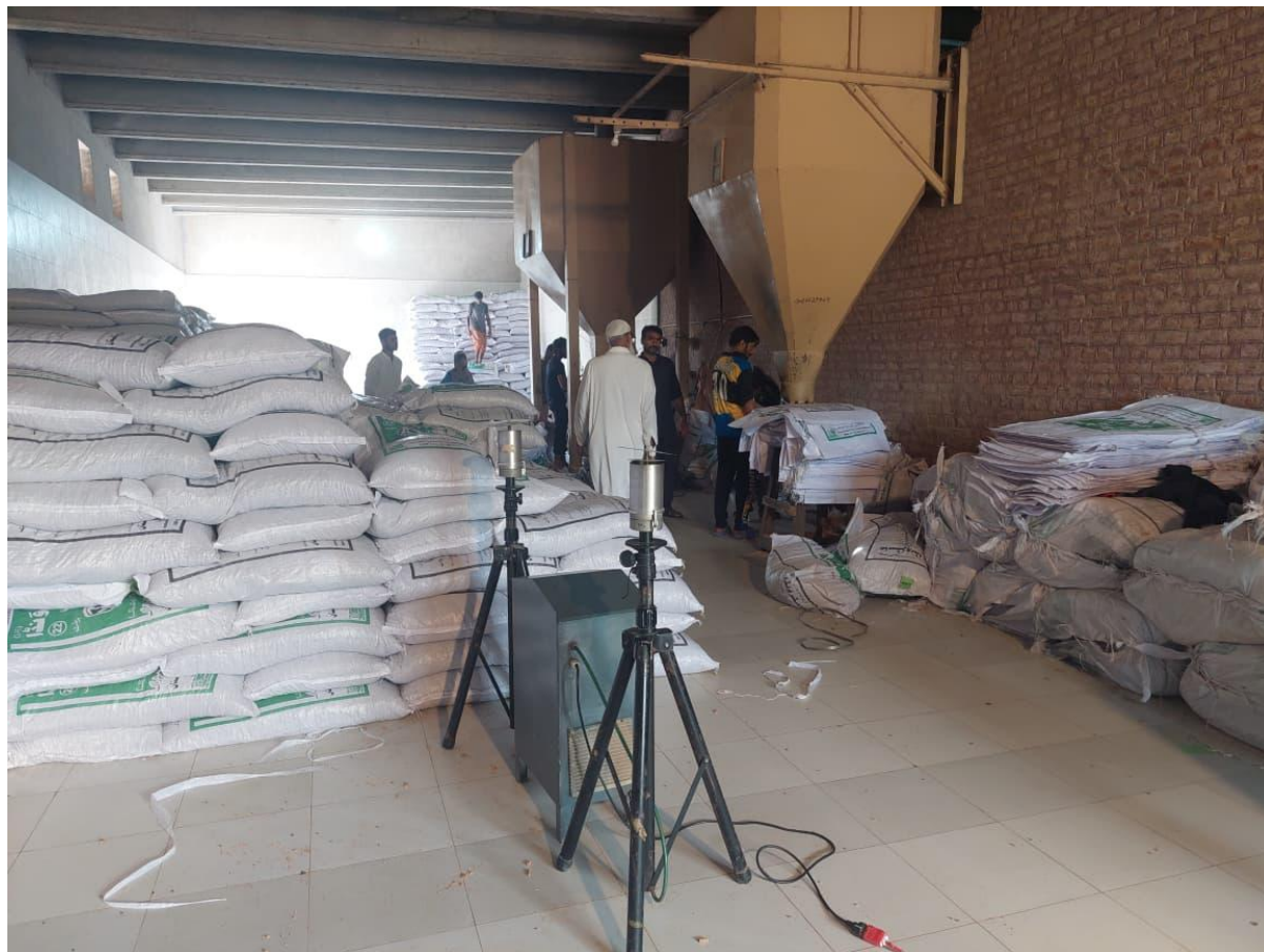
Figure 1 Particulate Matter sampling at the feed dispatch site.
