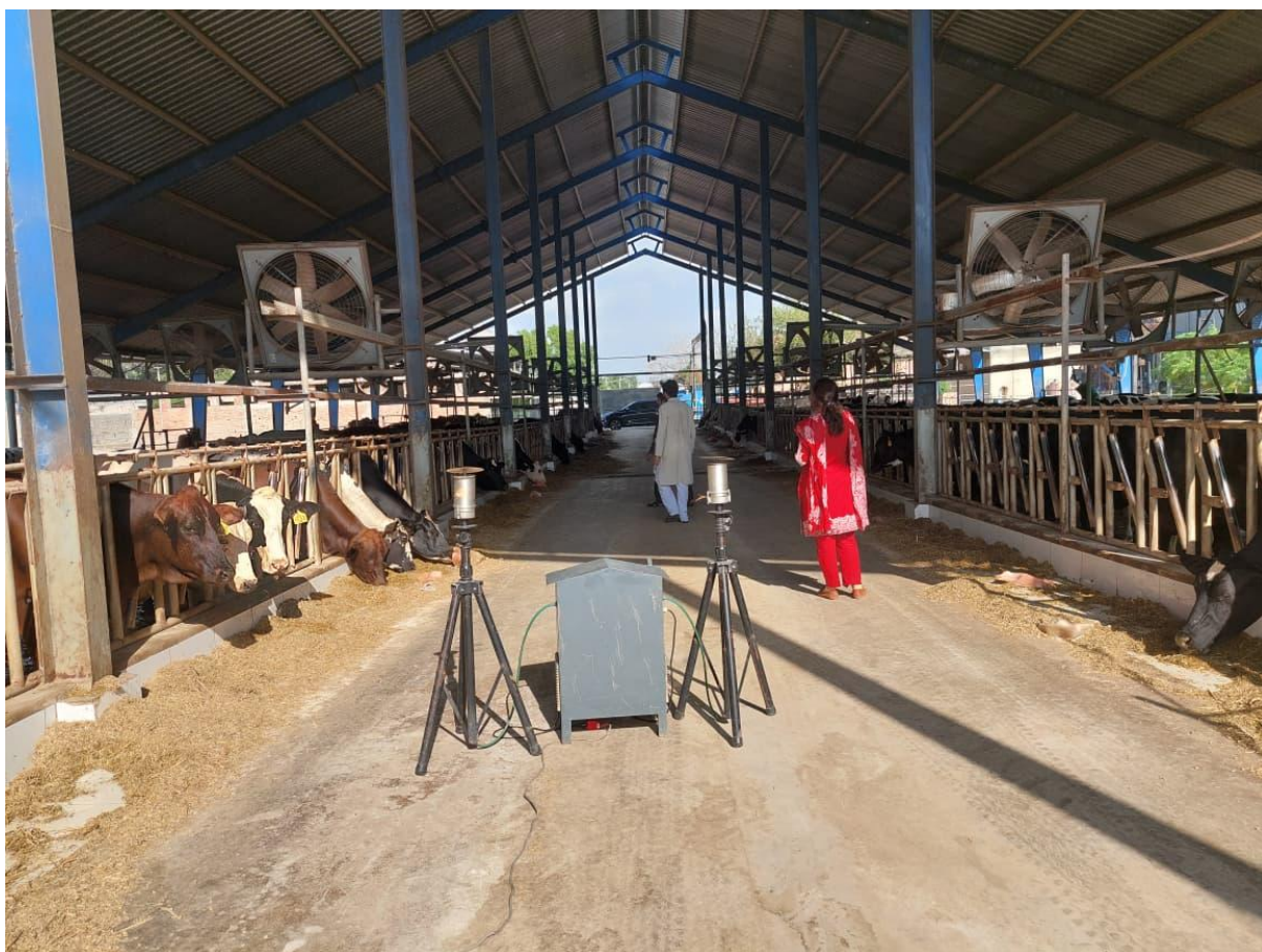
Figure 3 Particulate Matter sampling at Cow Byre site.
