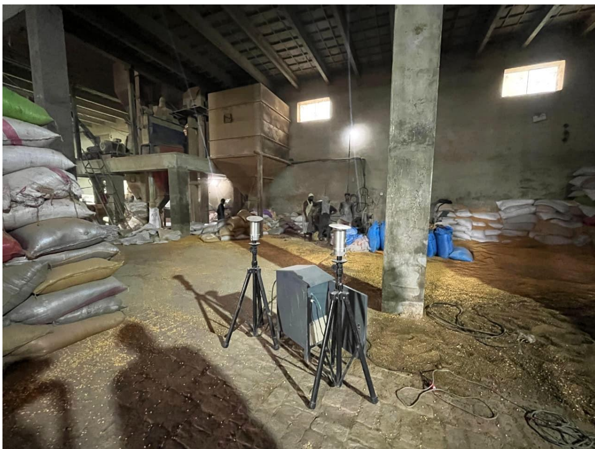
Figure 2 Particulate Matter sampling at feed manufacturing site.
