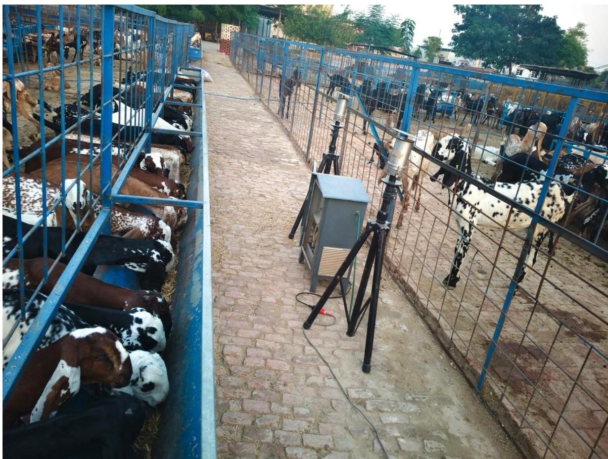
Figure 4 Particulate Matter sampling at Goat Pen site.
