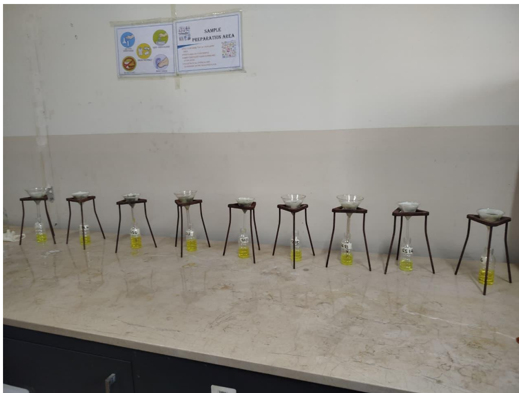
Figure 3.5: Sample Filtration Process
