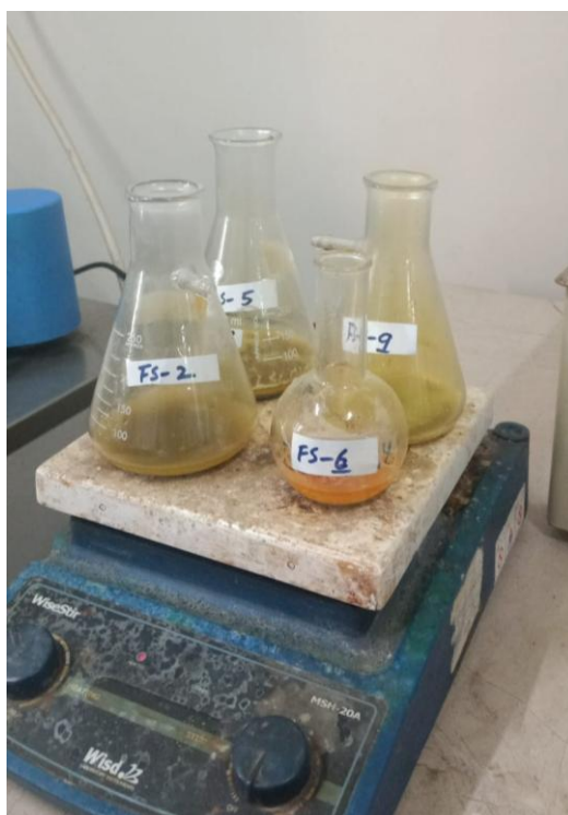
Figure 3.11. Heating sample solution for digestion of specimen fines in aqua regia
