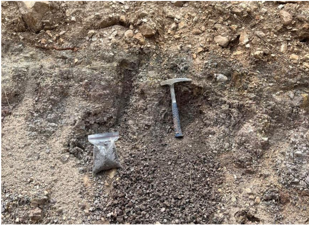
Figure 3.4. Field photograph of a weathered exposure of the Sardhai Formation at KRSS, Salt Range, showing its characteristic fine-grained, thinly bedded clay dominated lithology. A geological hammer is placed for scale and being used for collection of clay specimens. Representative specimens from fresh surface were collected from this section and stored in bags as shown for subsequent ICP-MS geochemical analysis, camera facing (NE)
