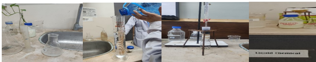
Figure 2.1 Preparation of stock solutions: (a) grinding tablets to fine powder, (b) dissolving powder in methanol, (c) transferring to volumetric flask, (d) filtration through 0.45 \mu\text{m} syringe filter.
