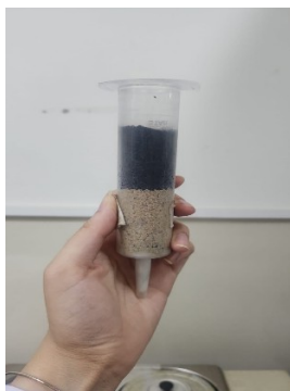
Figure 2.2 Packed fixed-bed adsorption column showing layers of cotton, 1 cm gravel, 4 cm silica sand, and 4 cm granular activated carbon (GAC) from bottom to top.
