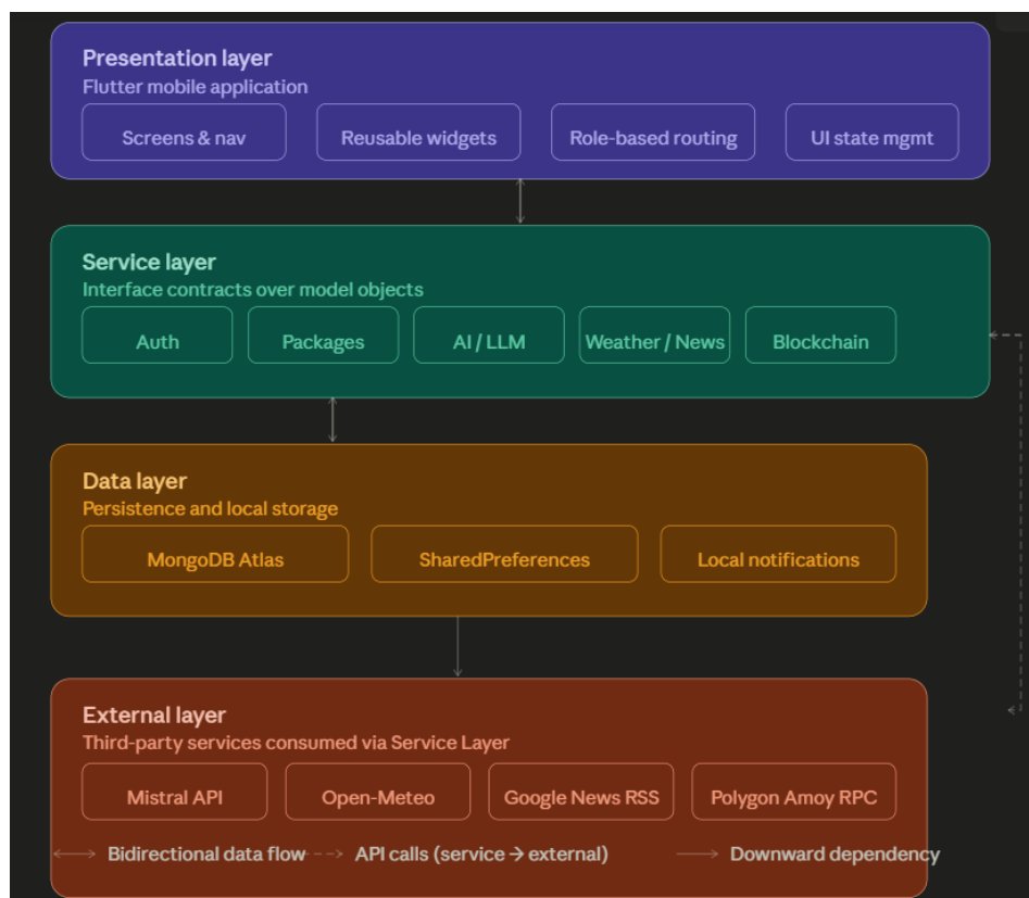
Figure 4.1: High-Level System Architecture – Four-Tier View
