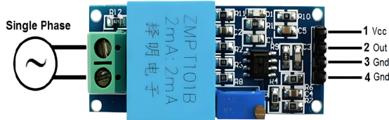
Figure 4.4: ZMPT101B Voltage Sensor
