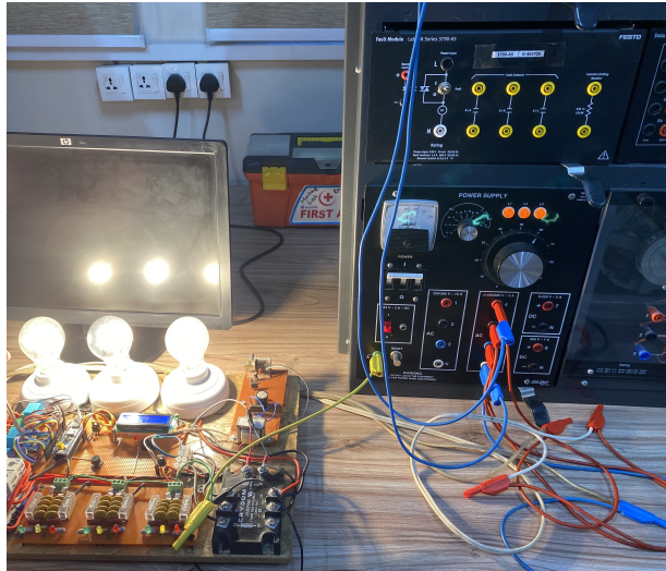
Figure 6.21: Installed System with Lab-Volt Three-Phase Supply
