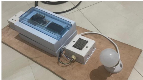
Figure 2.3: Lightning detection system with surge protection system
