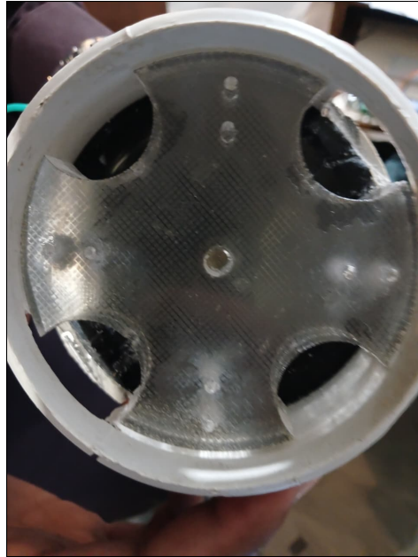
Figure 4.2: 3D-Printed Rotating Pocket-Wheel
