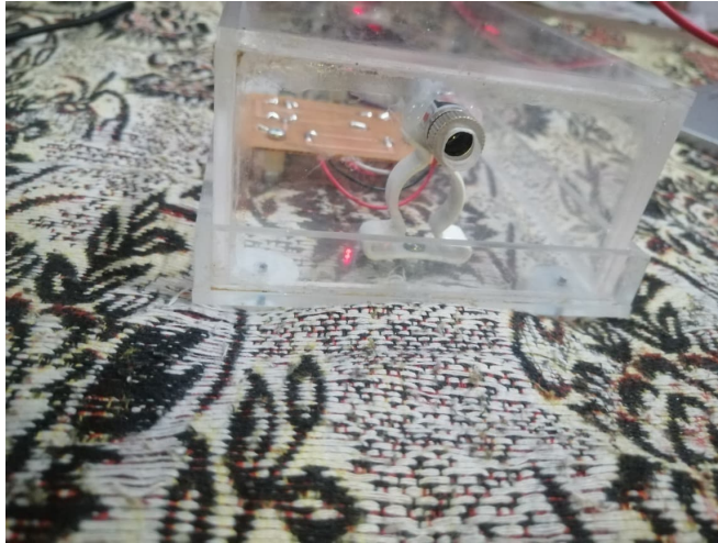
Figure 5.3: Li-Fi Transmitter Unit — front view showing laser diode output aperture and custom PCB circuit mounted inside acrylic enclosure. Red LED indicator confirms active power state during operation.
