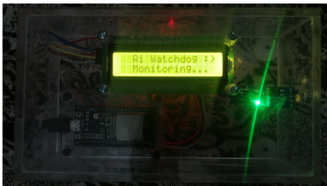
Figure 5.4: Li-Fi Receiver Unit in idle monitoring state — 16x2 LCD displaying “Ai Watchdog :) Monitoring...” confirming system is active and awaiting trigger. Green laser beam aligned with photodetector. Green LED status indicator illuminated.
