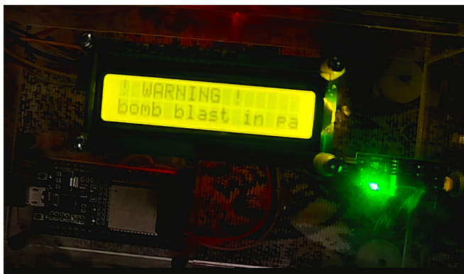
Figure 6.2: Li-Fi Receiver Unit in alert state — 16x2 LCD displaying WARNING message with detected trigger word received via optical transmission. Green LED illuminated confirming active alert. System auto-resets after 5000ms.
