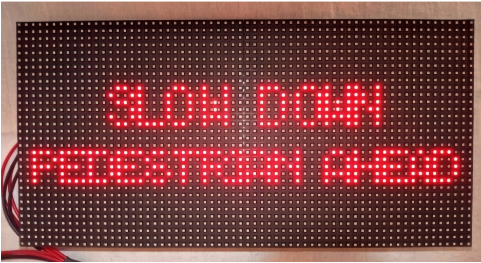
Figure 5.4: SMD LED display showing pedestrian warning message.
