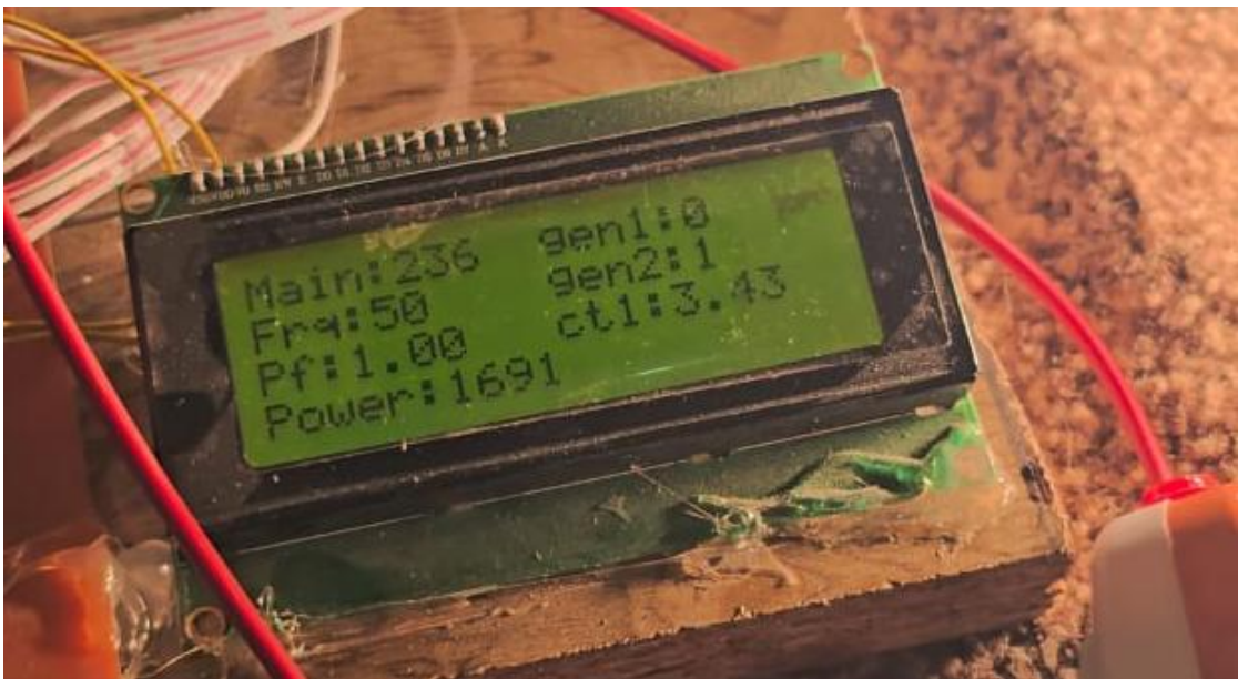
Figure 5.14: Hardware result when DG2 is ON
