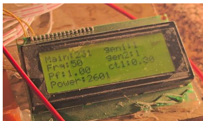
Figure 5.12: Hardware result when both DG's is ON
