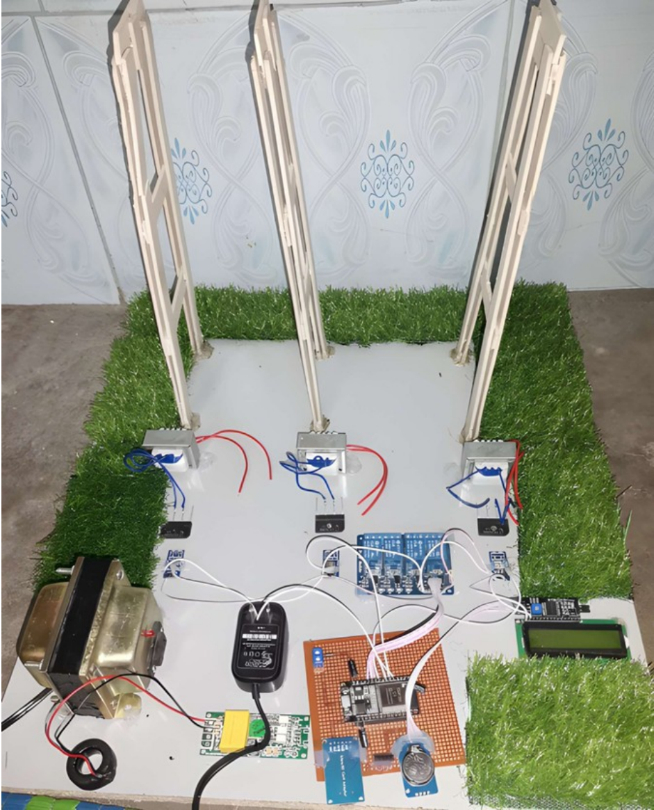
Figure 5.1: Hardware Implementation of the Grid Fault Detection Prototype.
