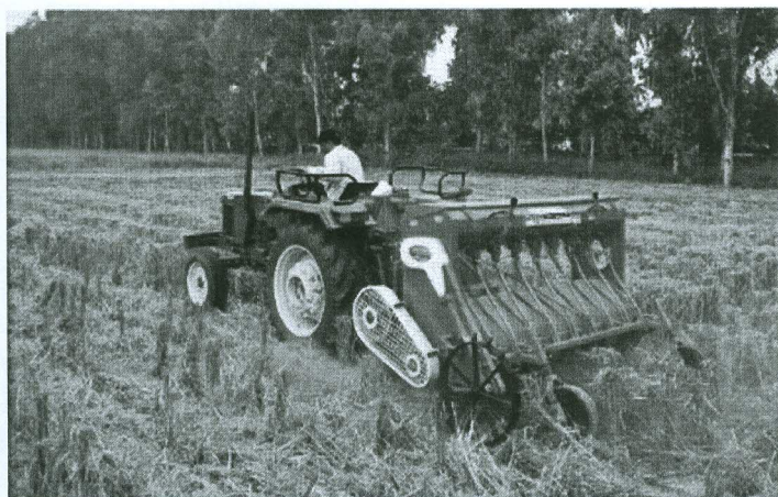
Figure 1 shows the operation of Happy Seeder
