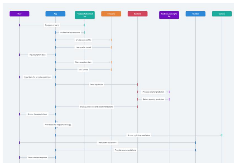
Figure 3.2: Aura-Soft Sequence Workflow Diagram
