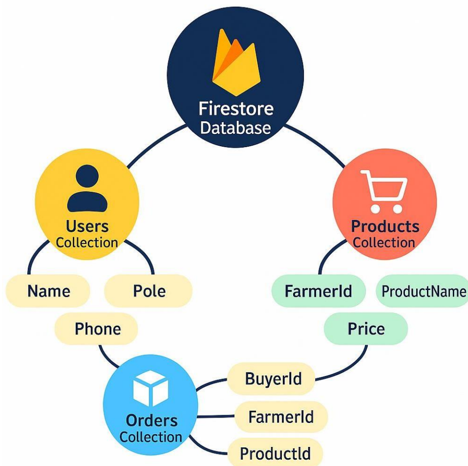
Figure 0.4: Firestore Database Structure
