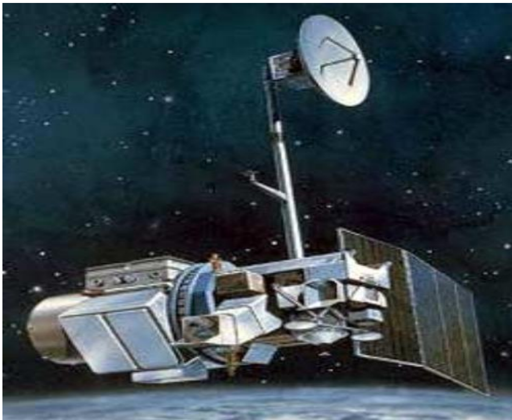
Figure 3.4 Landsat- 5 was launched in 1984. It supported the Multi Spectral Scanner and Thematic Mapper instruments [Image Source https://earth.esa.int/eogateway/missions/landsat ]
