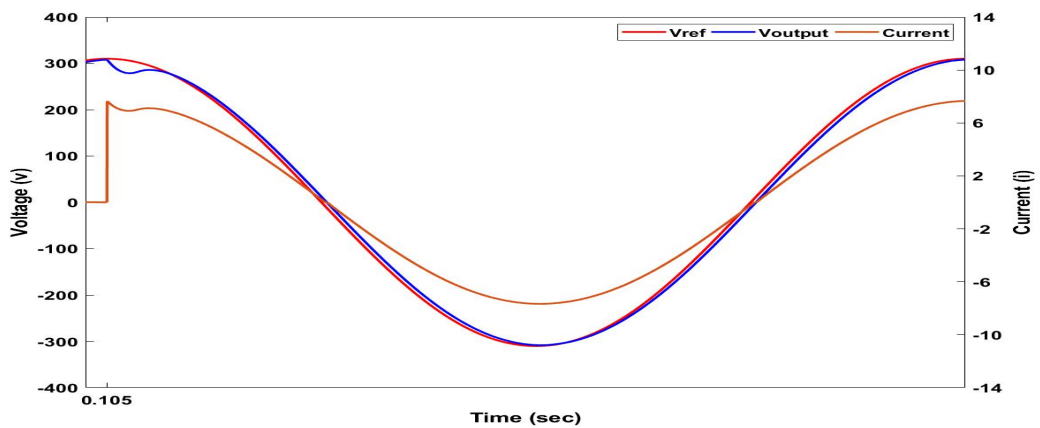
(c) Zoom: Transient response at 0.105 secs NL-FL condition (Transient response= 25ms).
