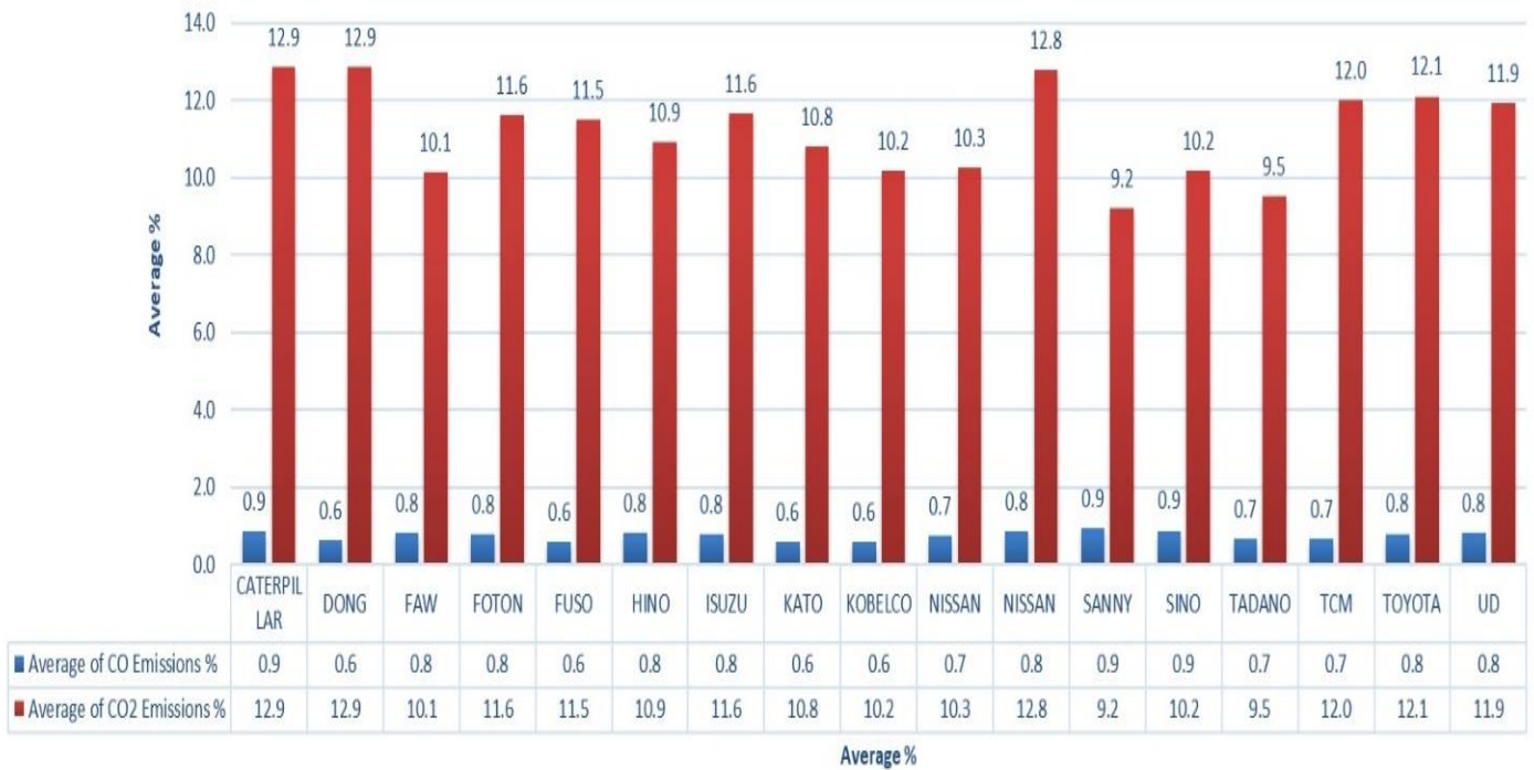
Figure 3.17 Emission Comparison by Vehicle Brand: Average CO and CO2 Levels for Diesel Engines
