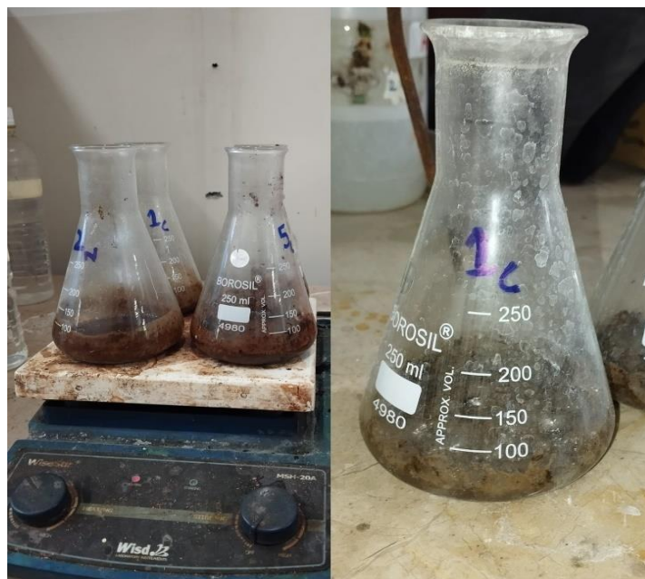
Figure 3.8 Soil digestion to prepare the sample for Zinc analysis.
