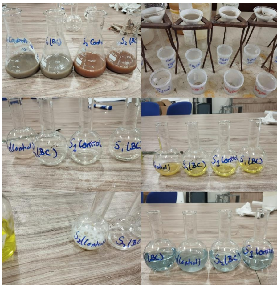
Figure 3.5 Sample preparation for phosphorus in soil.
