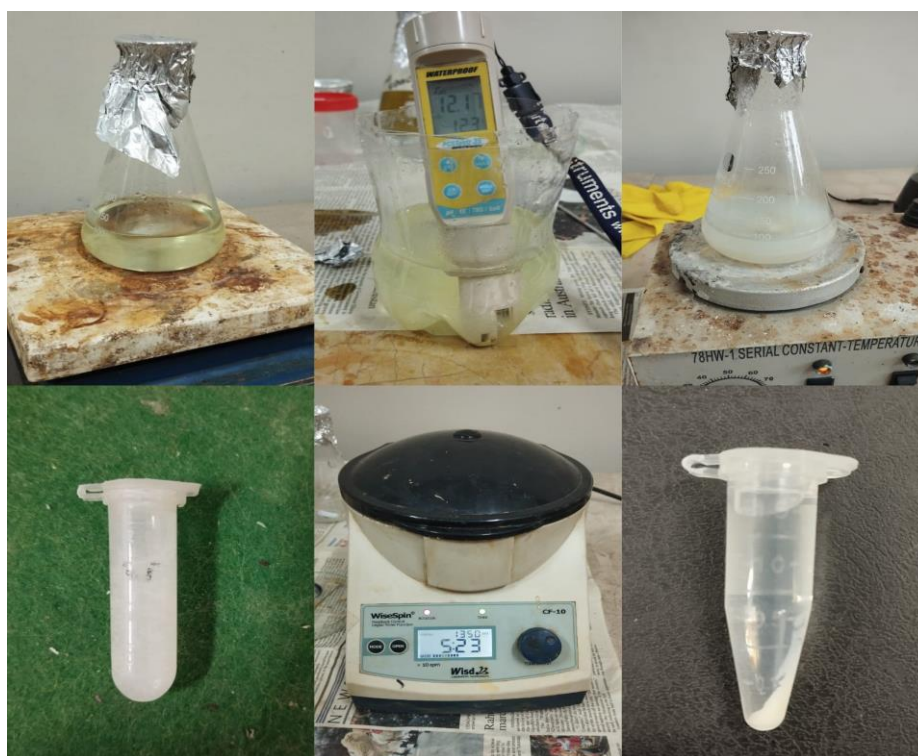
Figure 3.3 Preparation of ZnO NPs by Green-synthesis method.
