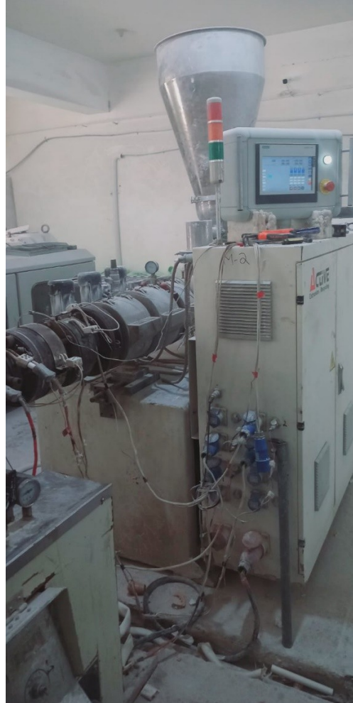
Extruder Feed hopper
