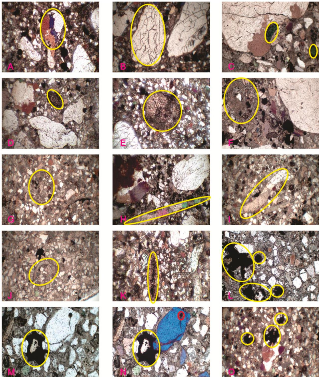
Figure 6.8 Microphotographs under XPL with 4X magnification, showing (A) polycrystalline quartz, (B) fractured quartz granules (C) tourmaline (D) algal fragment (E) bioclast (F) bivalve shell (G) gastropode (H) recrystallized calcite filled shell fragment (I, J) oyster shells (K) pyritized shell (L) pyrite cement (M) pyrite cement under (PPL) (N) pyrite grain on quartz granule and (O) pyrite cement with a polycrystalline granule in medium grained sandstone.
