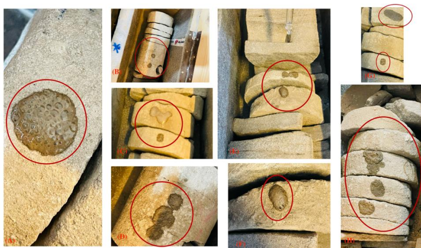
Figure 4.19 (A to H) Marked stains showing rigorous bubbling when reacted with 10% HCl due to the presence of calcareous material. Coarse to vary coarse grained brownish grey unconsolidated sandstone is visible.
