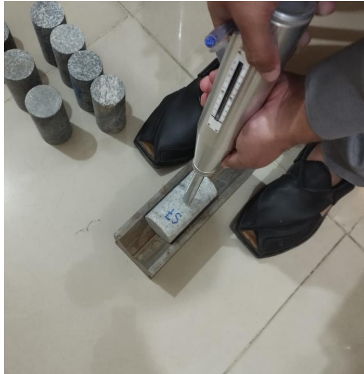
Figure 3.6 Performing Schmidt rebound hammer test (Sample 7)
