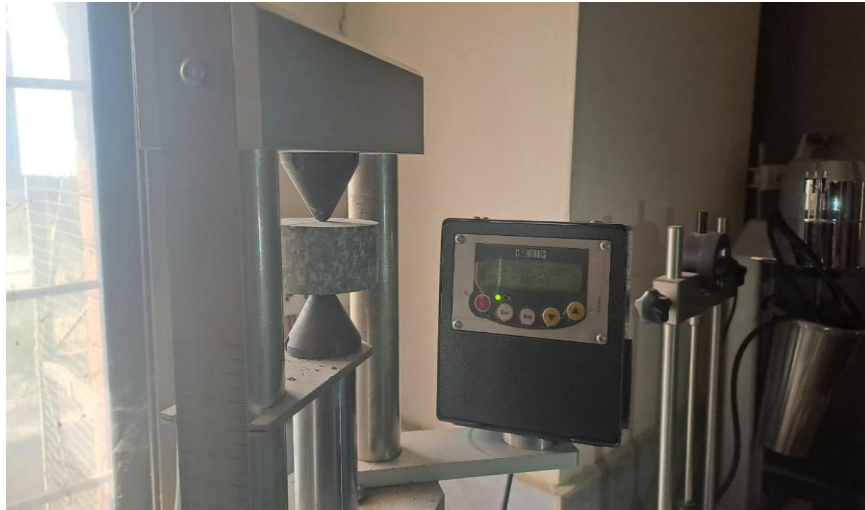
Figure 3.4 Point load test (sample 1)
