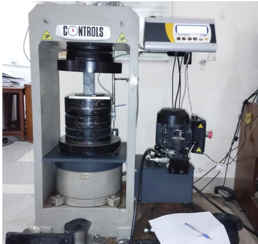
Figure 3.2 Unconfined compressive strength test (sample 1)
