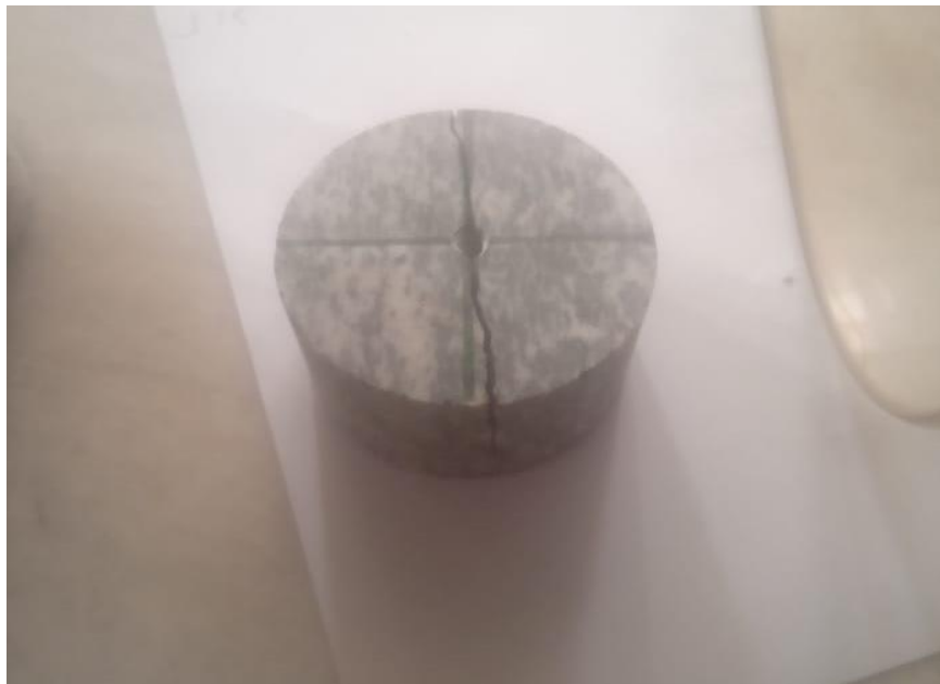
Figure 3.5 Sample 1 after point load test
