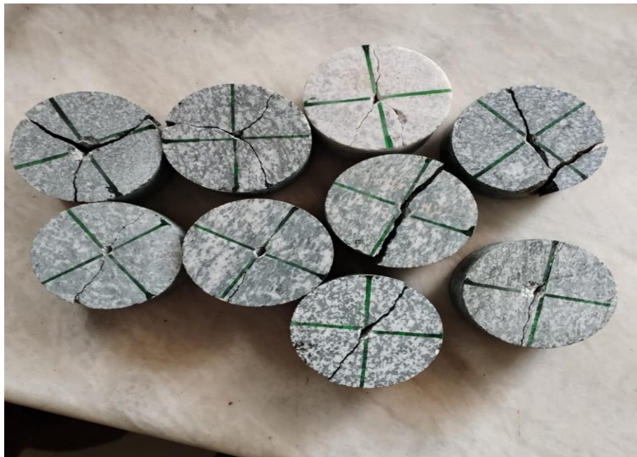
Figure 3.3 Samples after UCS test
