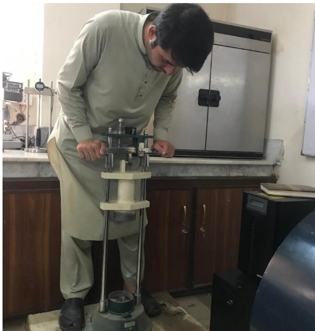
Figure 3.7 Aggregate Impact test
