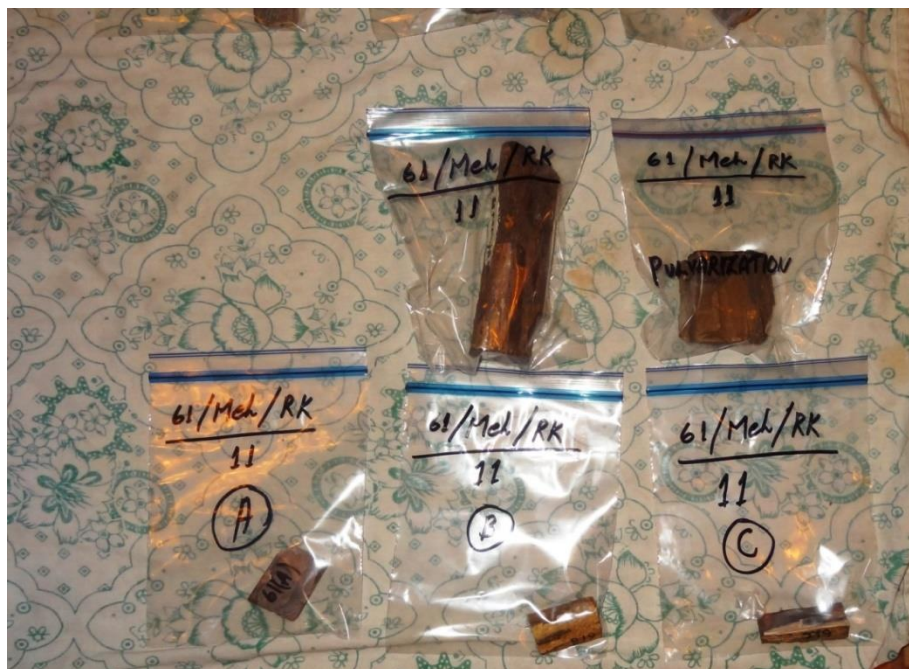
Figure 3.14 Cutting of each wood fossil specimen into three dimensions and specified section for 13C analysis (pulverization)
