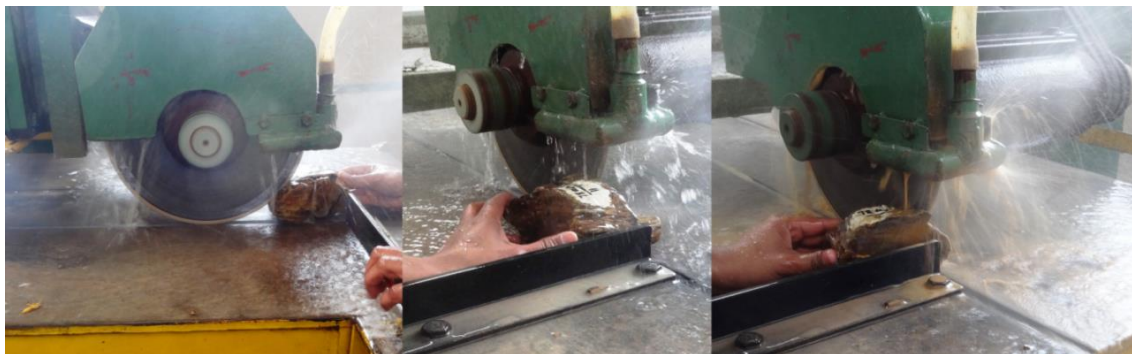
Figure 3.11 Cutting of wood fossils in three dimensions
