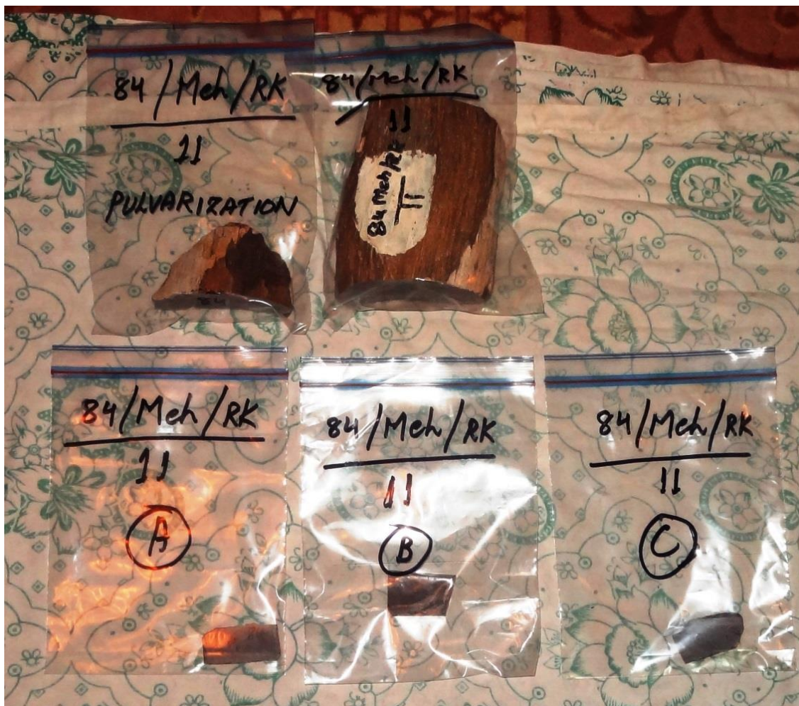
Figure 3.15 Cutting of each Wood Fossil specimen into three dimensions and specified section for ^{13}\text{C} analysis (Pulverization)
