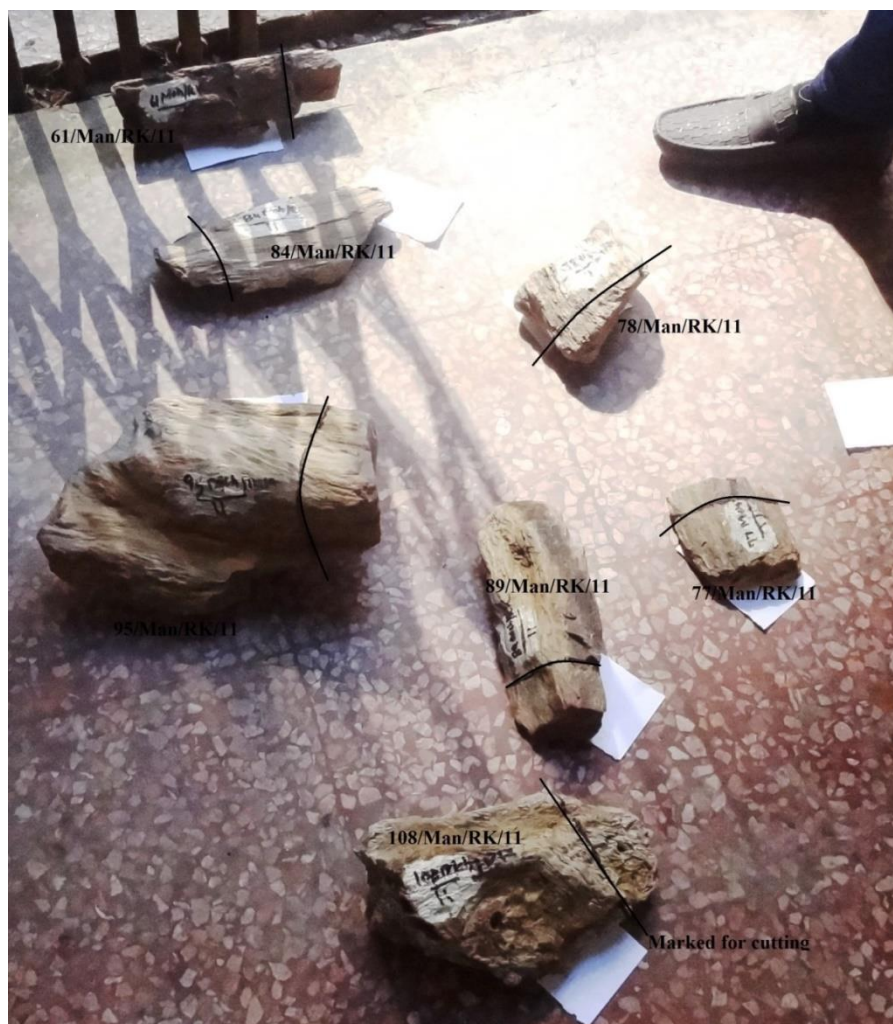
Figure 3.8 Petrified wood fossil specimens marked for cutting for making slabs for thin sections
