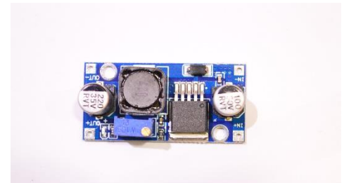
Figure 4: Dc Step Down Variable Voltage Regulator
