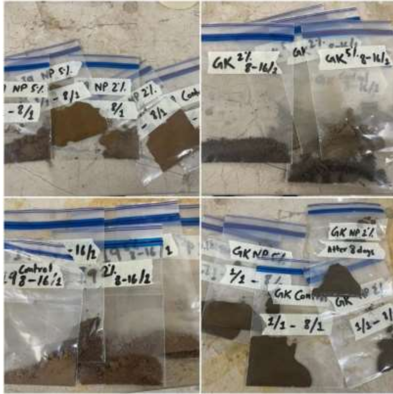
Figure 2.6: Prepared twenty samples of the soil for heavy metal analysis
