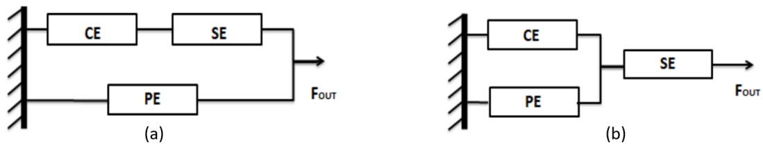
Figure 4 a) Block diagram of 1st Hill model. b) Block diagram of Alternate Hill model.
