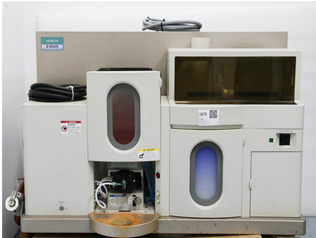
Figure 8: Hitachi Model Z-2000 atomic absorption spectrophotometer (Adler et al., 2019).
