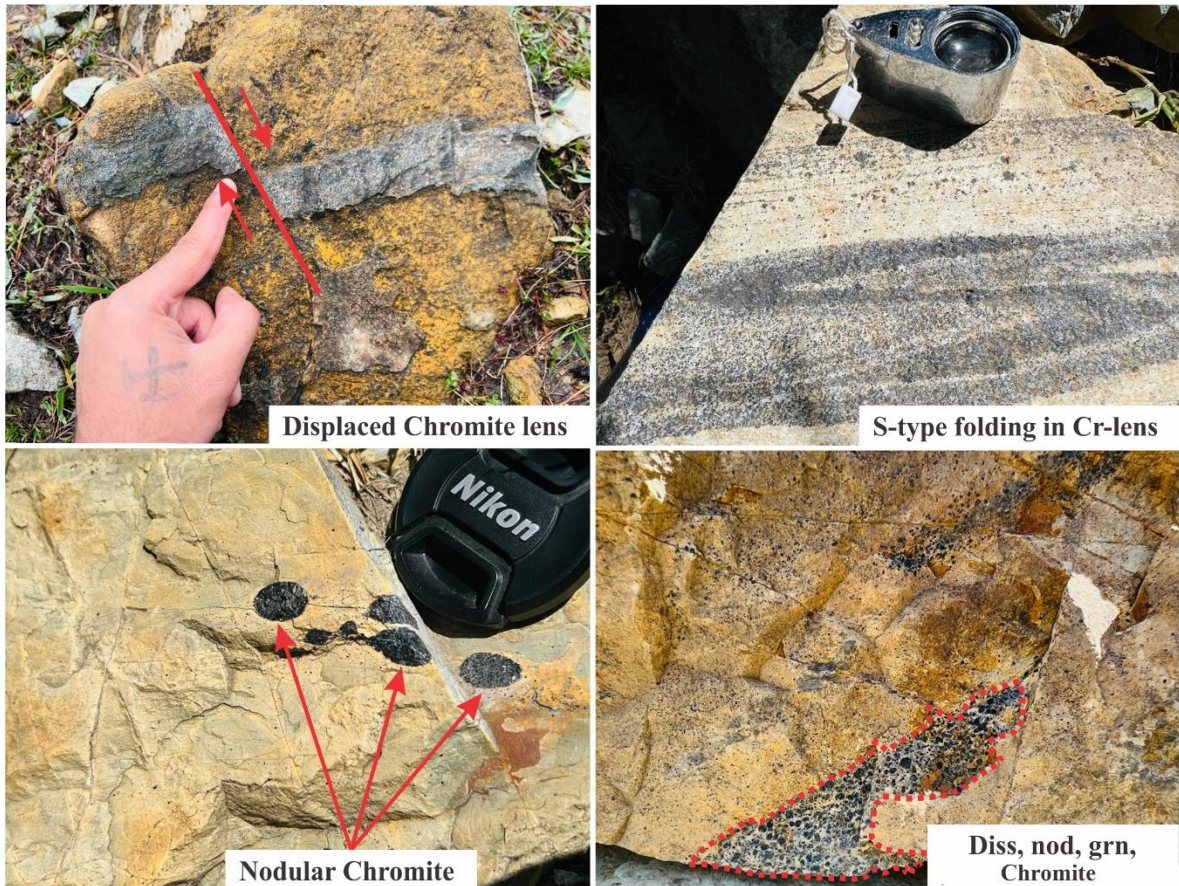
Figure 3.18 (a) Displacement of chromite lens (b) S-type folding in chromite lens (c) Nodular chromite in dunite rocks (d) (Diss) Disseminated, (nod) nodular and (grn) granular chromite in dunite body
