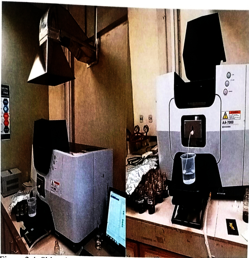
Figure 2.4. Shimadzu Atomic Absorption Spectrophotometer (AA-7000 Series)
