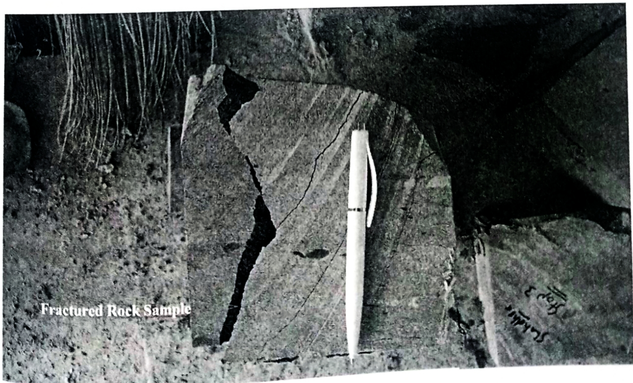
Figure 4.2 Fractured rock sample after UCS test
