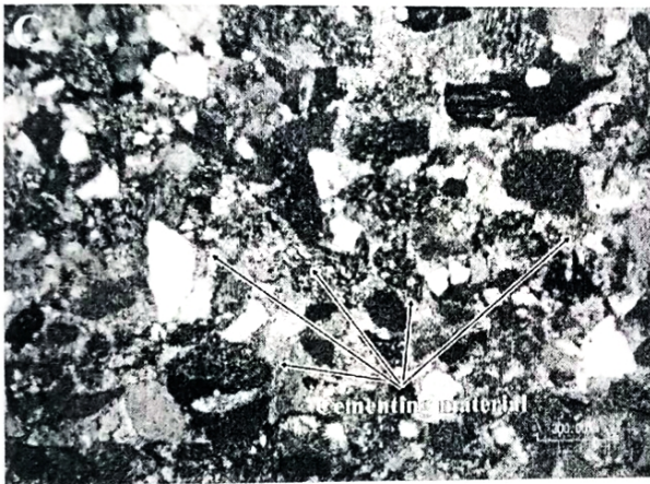
Fig 3.5. A (XPL) showing iron ore, B (XPL) showing various rock fragments i.e. sedimentary and metamorphic, C (XPL) showing cementing and matrix material, D (XPL) showing metamorphic rock fragment(quartz-mica-schist)
