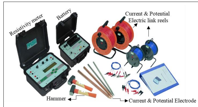
Figure 4.2 The instrument used for data acquisition PASI-Earth (16-GLN) resistivity equipment.
