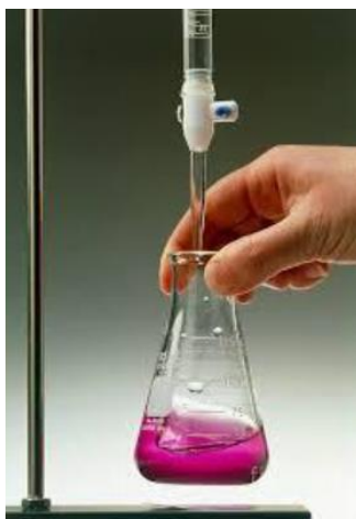
Figure 3.9 Titration for Ca and Mg
