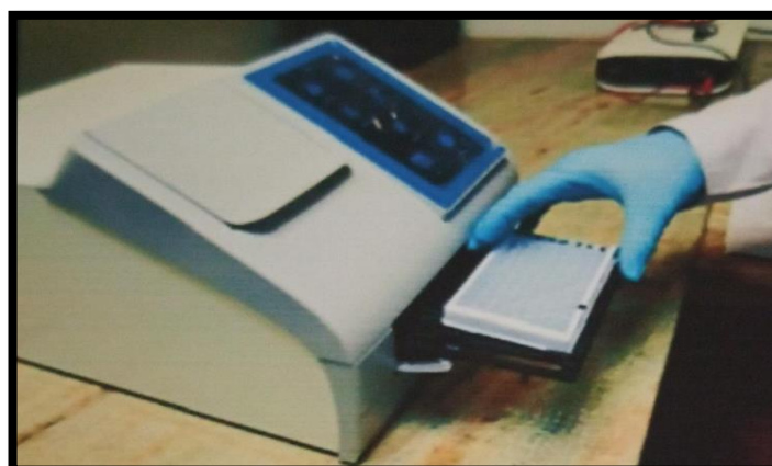
Figure 3.7(d): sCD40L; Sixty minutes of sample incubation of done in Spectrophotometer at 37 o C.
