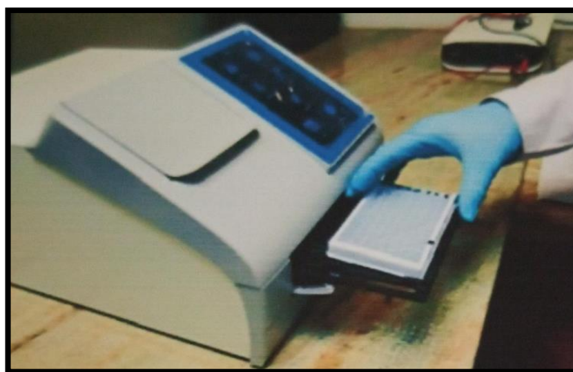
Figure 3.6 (d): MCP-1;Sixty minutes of sample incubation of done in Spectrophotometer at 37 0 C.
