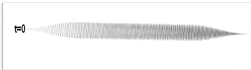
Figure#17: Vibroseis wavelet. (Yilmaz, 2001)
