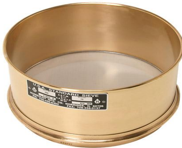
Figure 4.2: Wet wash sieve with mesh opening No. 200
