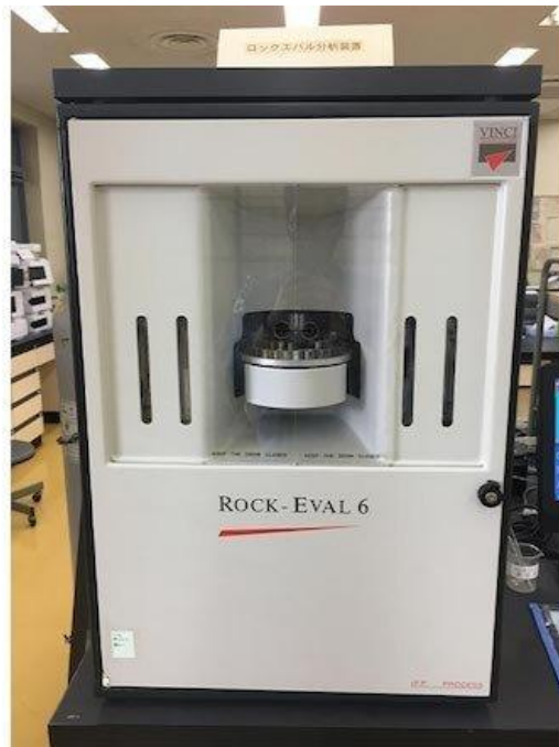
Figure 3.6 Rock Eval 6 used for determination of S1, S2, S3, and T max
