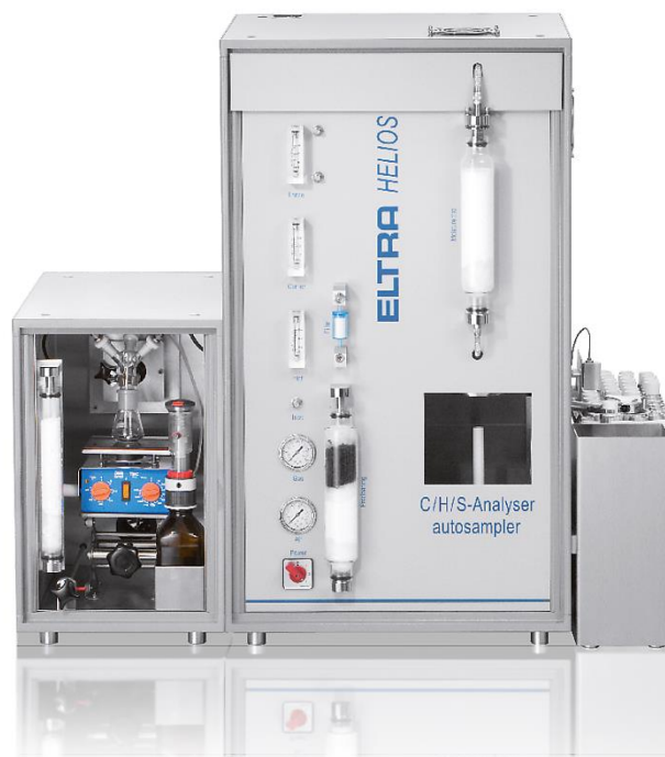
Figure 3.5 Carbon and Sulfur analyzer CS-580 A (Helios) used for determination of TOC
