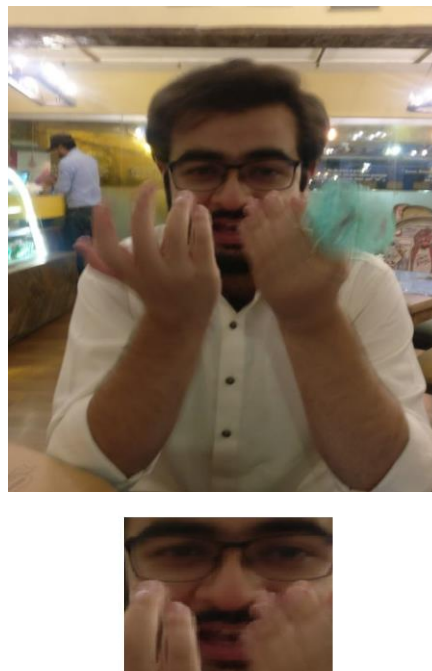
Figure 3.8: Face Detection on blurred image using Dlib A face that is being covered by hands can be detected with Dlib. This can be seen in Figure 3.8. Blurred faces can also be detected.
