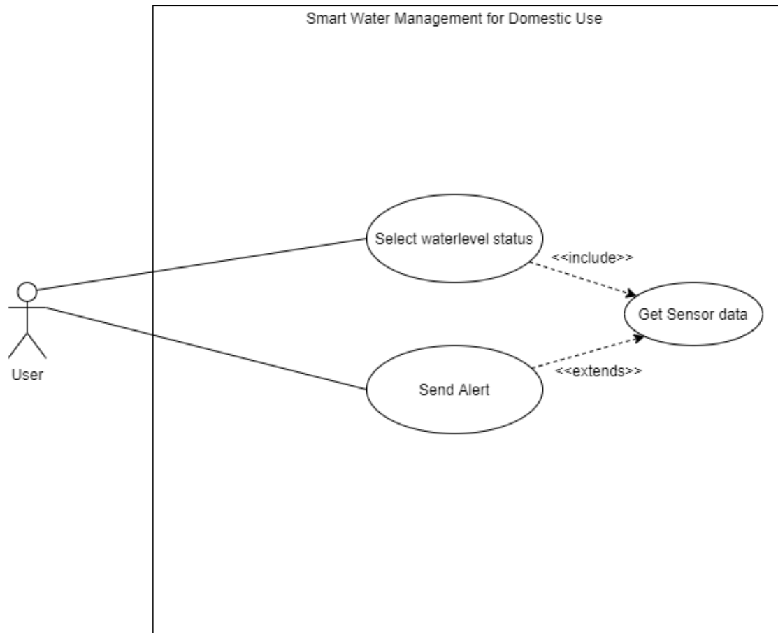
Figure 3.3: Use case 2 - Check Water Level
