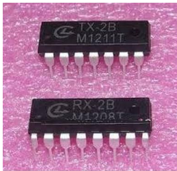
Tx2b and Rx2b IC is used for five channel radio remote control circuit Fig 3.13
