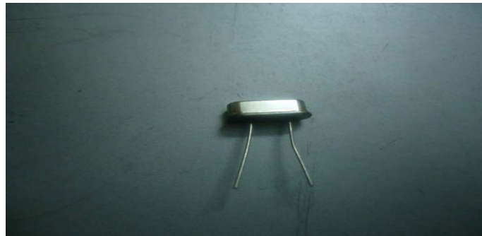
Figure 10 (chapter 2) simple oscillator
