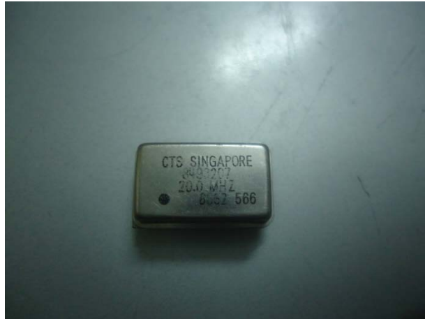
Figure 11 (chapter 2) High speed oscillator
