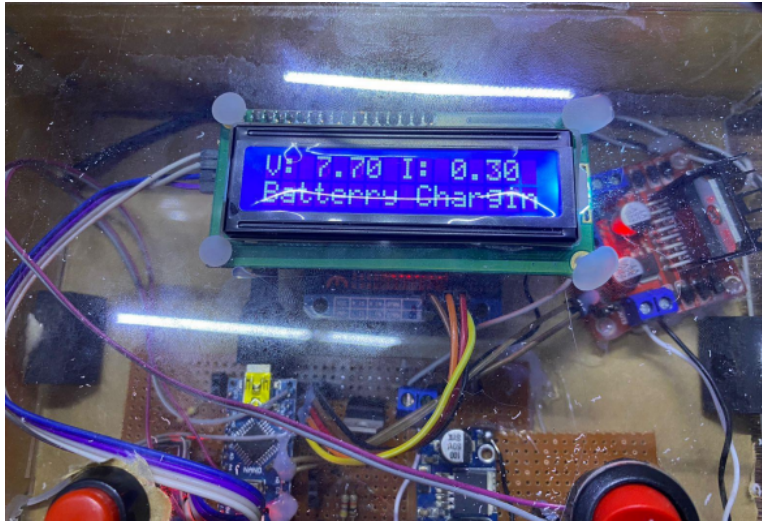
Figure 5.1: LCD during battery charging mode.
