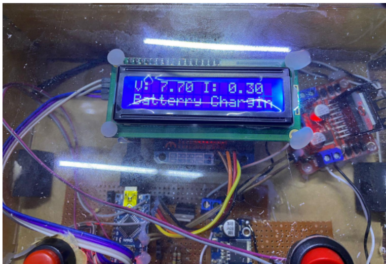
Figure 6.1: LCD during battery charging mode.
