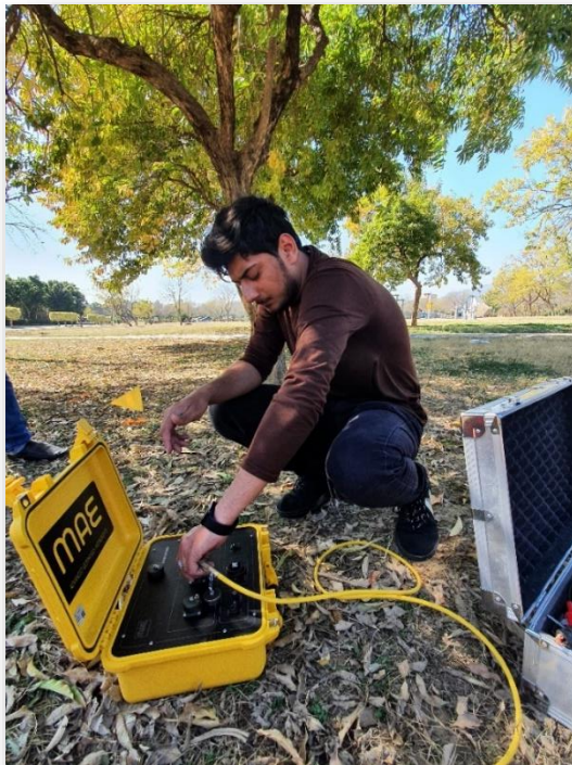
Figure 3.7. Connecting wire of first channel with seismogram similarly second channel will be connected to seismogram and then connecting wire of triggering geophone will be connected to seismogram
