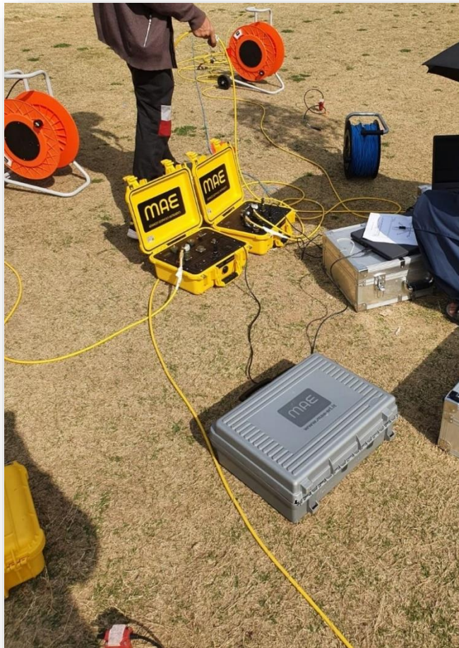
Figure 3.3. Setting up instruments in field in which two seismographs have been connected with two channels while triggering geophone is been connected with seismogram
