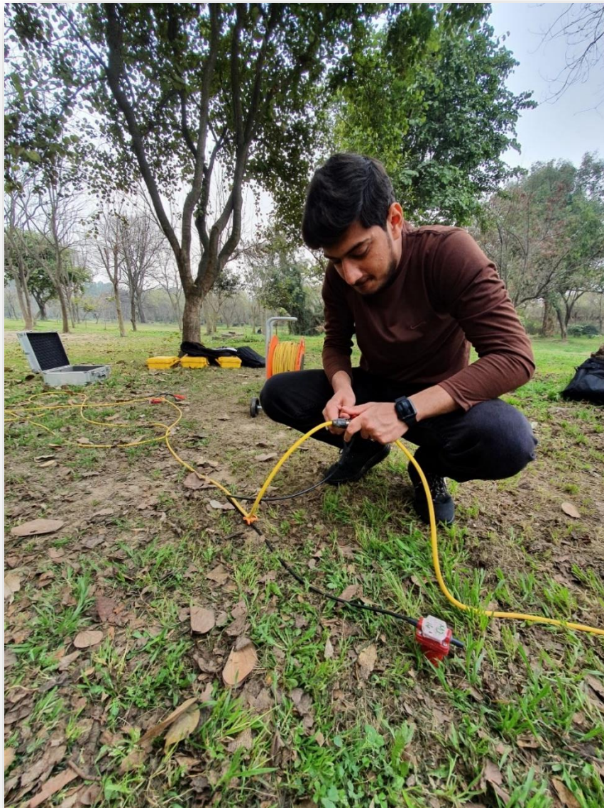
Figure 3.4. Connecting positive and negative terminal of geophones with connecting wire which is then connected into seismogram in the field
