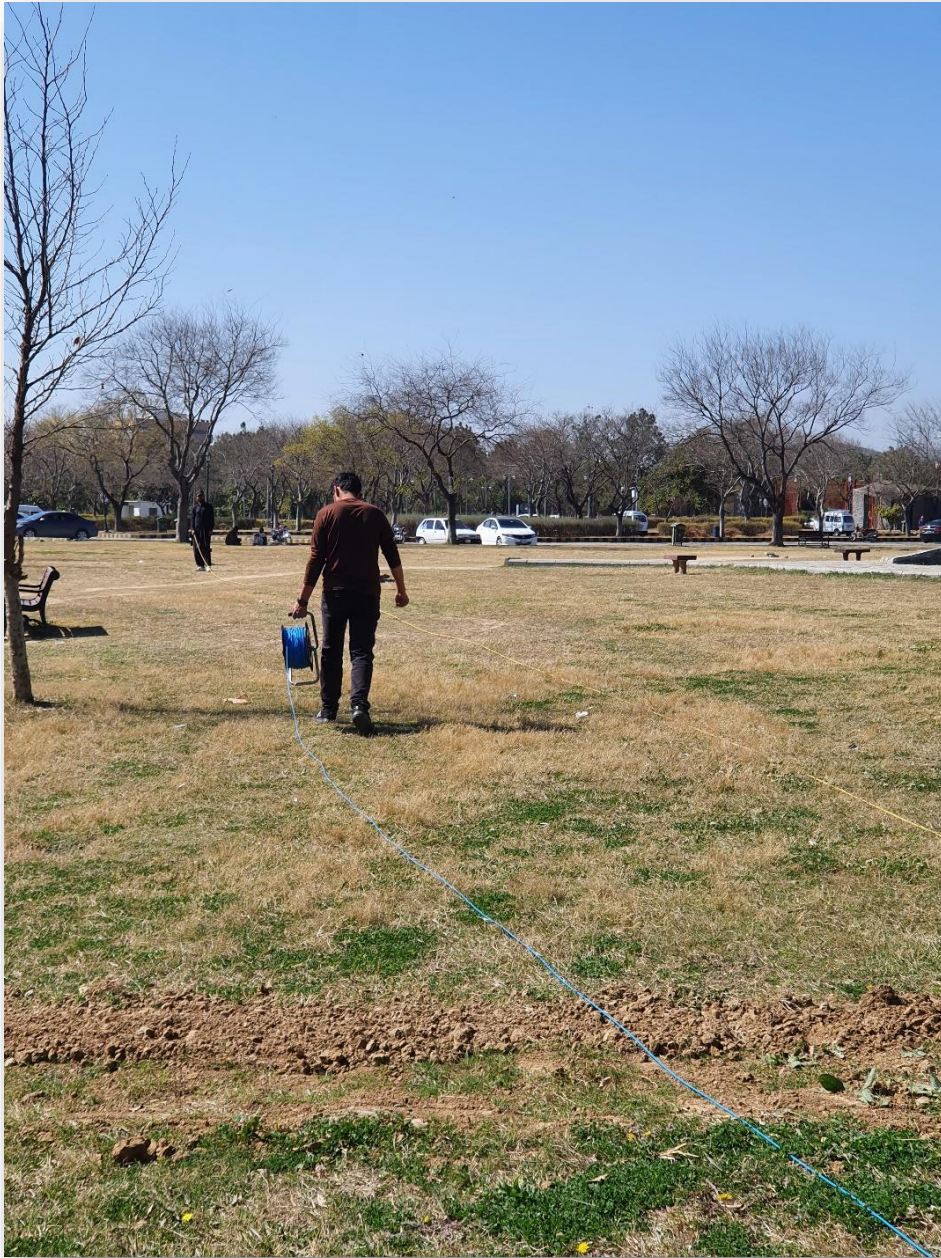
Figure 3.16. Setting up connecting wire for triggering geophone for MASW survey at 2nd site, its one end is connected with triggering geophone and other end with seismogram
