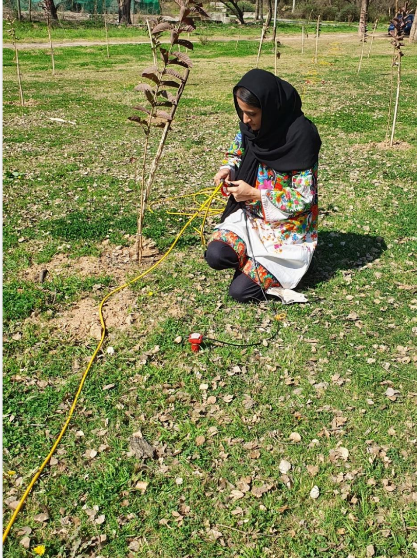
Figure 3.19. After setting geophones connecting positive and negative terminals of geophones with connecting wire
