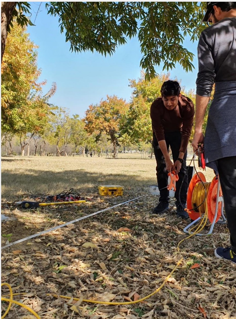
Figure 3.9. Measuring distance using measuring tape between two geophones to keep spacing between two geophone to 5 meter
