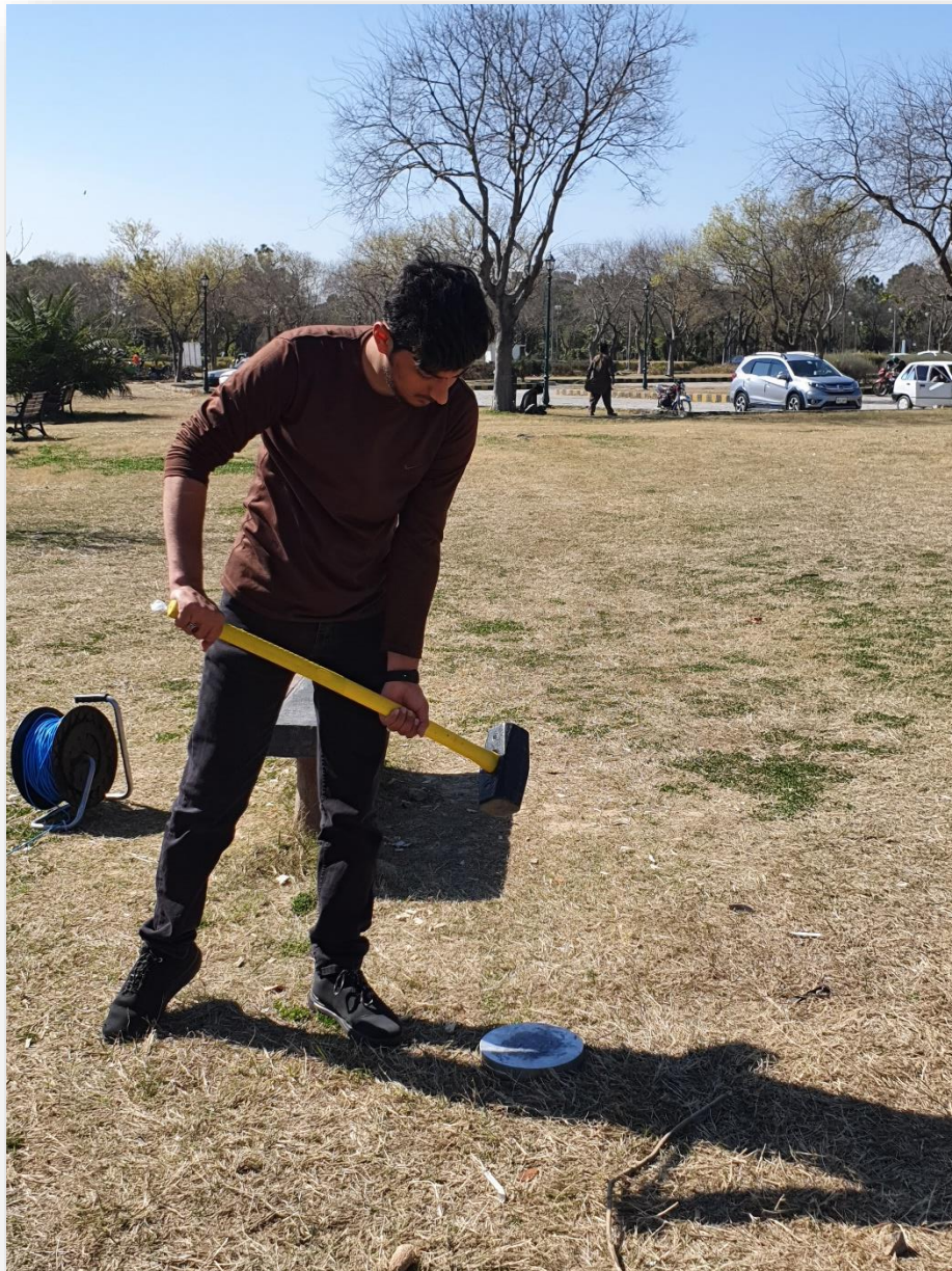
Figure 3.10. Taking shots by striking hammer with metal plate for MASW survey
