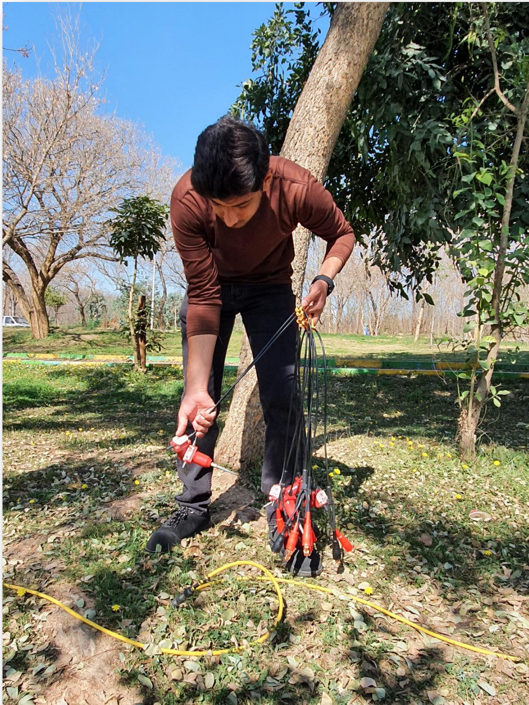
Figure 3.15. Spreading Array and setting up geophones for MASW survey at site 2 after which their positive and negative terminals are connected with connecting wire which is then connected into seismogram
