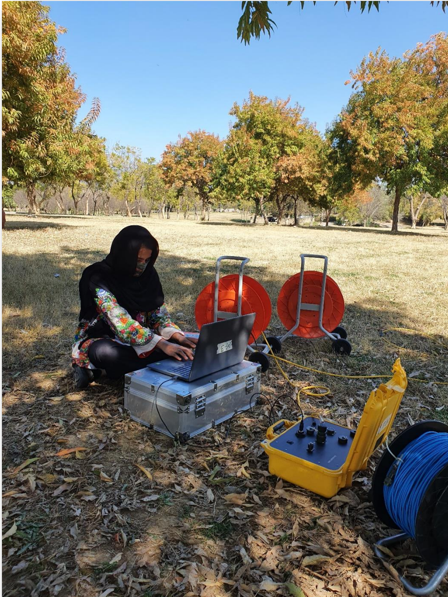
Figure 3.8. Running Geophone Test in Field before survey to make sure all geophones are properly connected and working properly and recording the traces
