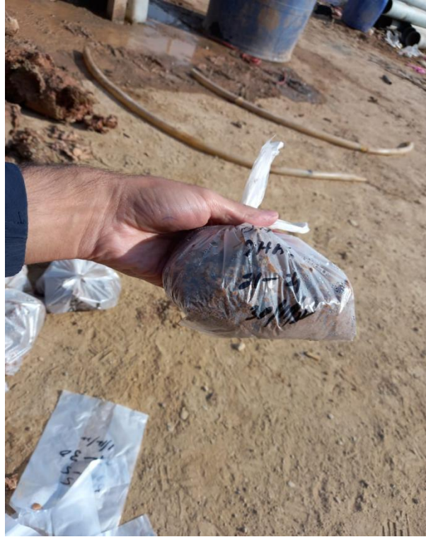
Figure 4.3. Samples from BH-4 being put in the polythene bag to maintain moisture.
