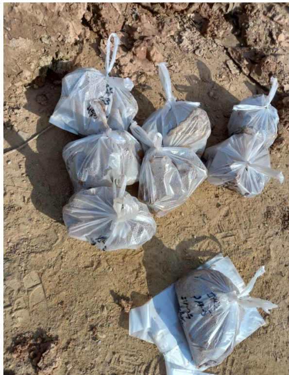
Figure 4.2. Samples taken out from SPT test at BH-4 depth 6m.
