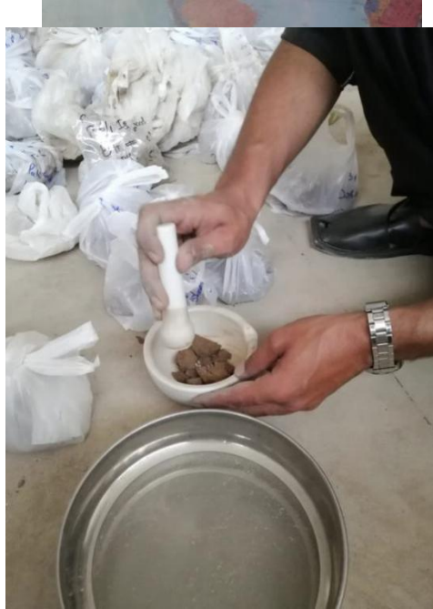
Figure.4.6. Using pestle and mortar to crush the lumped soil.
